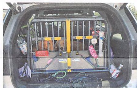
For dogs who aren't properly crate trained, the VarioGate system (top photo) adds a layer of crash-tested protection for your dog and protects you from your dog becoming a dangerous flying object during a crash. The VarioCage (bottom) also offers a very airy look that may suit non-crate-loving dogs.
