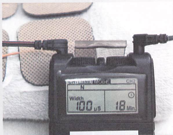
There are a variety of TENS units on the market, but they all consist of electrodes (in back) and a monitor.
